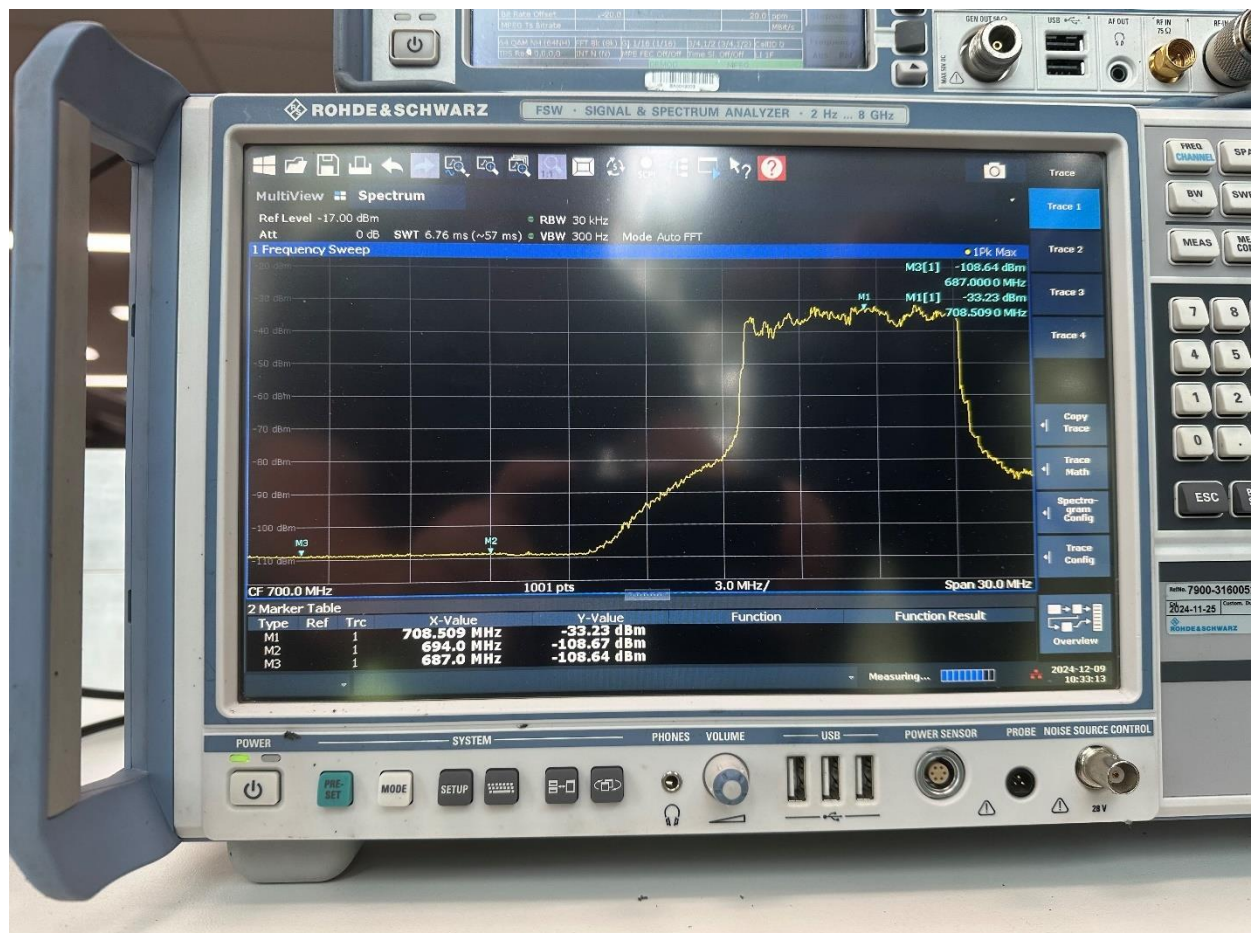
Figure 2 – OOB/E Measurements of a UE device conducted at Freeview Labs
